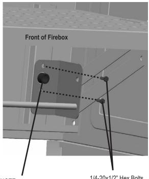
NOTE: Mounting bracket with hole fits over threaded bushing
